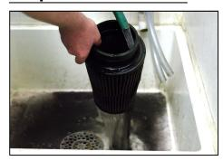
Rinse off air filter with cool low-pressure water from the inside out, in order to flush the dirt out of the filter. Continue to rinse the filter until all traces of cleaner are gone, and water runs clear through filter. It may be necessary to repeat steps 1 and 2.
