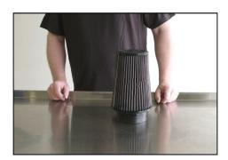
After rinsing, gently shake off excess water and allow filter to dry naturally. Do not apply the oil until the filter is completely dry.
