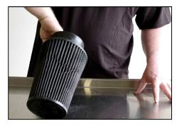
Remove any large debris from the filter prior to application by tapping GENTLY against hard surface.
