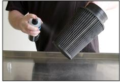
Liberally spray Cold Air Inductions Air Filter Cleaner on both sides of filter and allow to soak for 10 minutes to loosen the dirt. Do not allow cleaner to dry on air filter.
