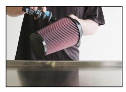
Touch up any light areas on either side of the filter until there is a uniform red color on all areas. Allow the filter to sit for 24 hours. Wipe off any excess oil at filter base.
