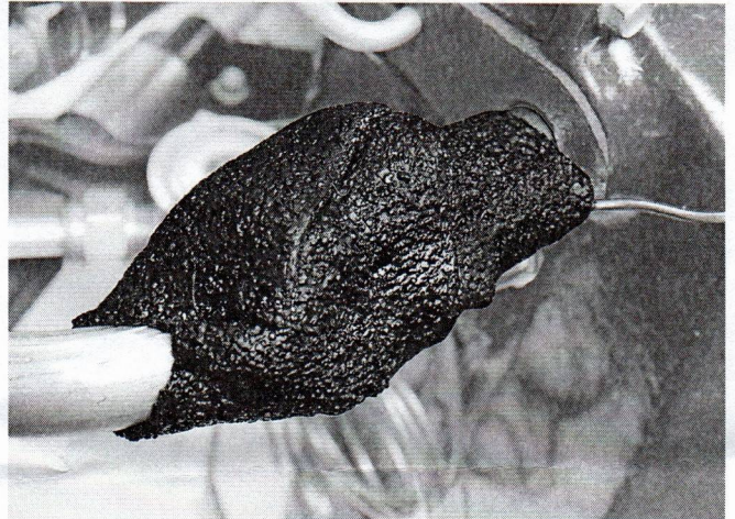
Photo 3 - Wrap Sensors with Insulating Tape
