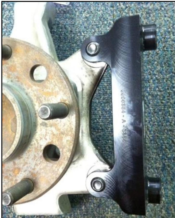
**Figure 1:** Base bracket installed onto spindle
