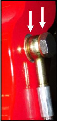
**Figure 5:** Installation of hose and washers
