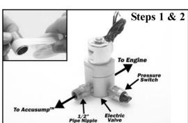
\*WARNING\*\* Do not use the valve solenoid as a handle for installation. Use a wrench. Bent valve shafts and damaged solenoids due to improper installation are not covered under warranty.
