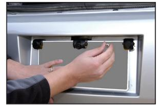
Secure license plate bracket with provided screws
