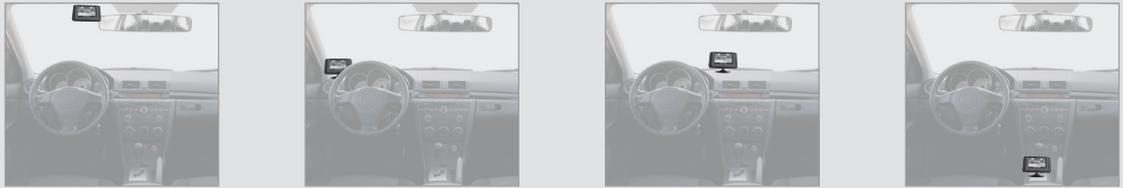
Place monitor (A) in desired location (dash or windshield) (Fig. 1) but do not permanently mount until later.
