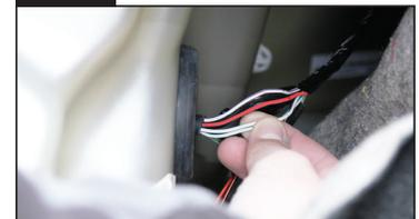
Locate the reverse light wire and splice the red wire to the reverse light wire
